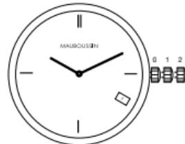
Pull the crown initially in position 0 to position 2. Set the hour and minutes hands. Do not forget the crown back to position 0.
